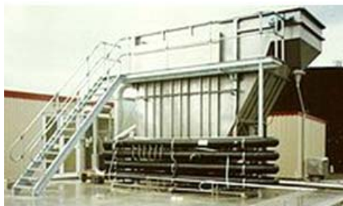
Fig.15: Dissolved air flotation system for treating industrial wastewater ( http://en.wikipedia.org/wiki/file:redox-daf-unit-225-m3-h1000-gdm )
