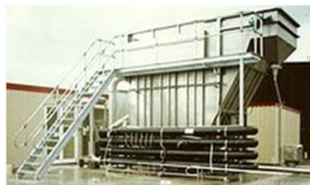
Fig. 14: Dissolved air flotation system for treating industrial wastewater, ( http://en.wikipedia.org/wiki/file:redox-daf-unit-225-m3-h1000-gdm )
