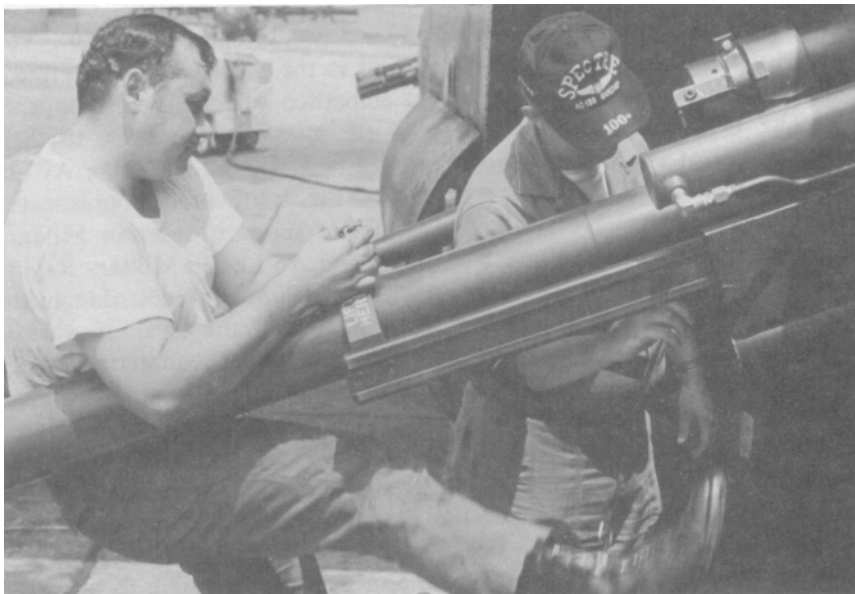
Top: Crewmembers steady a 105-mm howitzer during installation into an AC-130H; bottom: Personnel of the 16th SOS mount a 105-mm howitzer in an AC-130H.
