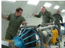
Capture Basket concept testing on NASA C-9 zero-g aircraft
