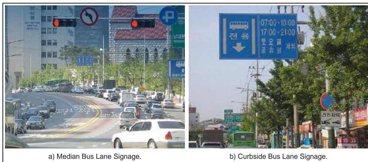
Figure 32. Bus Lane Signage Examples (Seoul)
