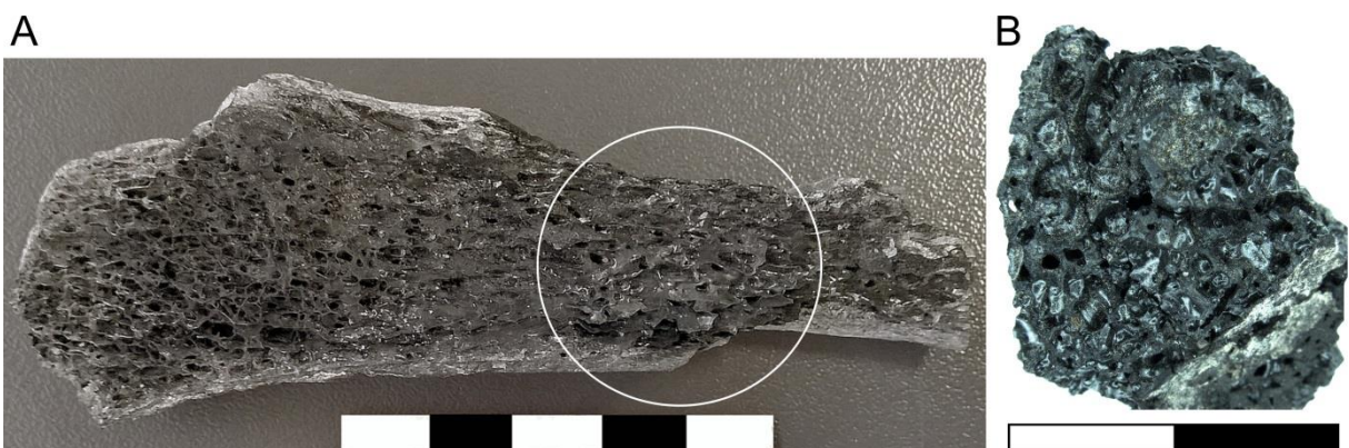
Figure S6 - Glassy appearance in bone and charcoal. A. Trabecular bone characterized by an intact structure with partial glassy appearance (white circle) (left tibia, human victim's skeleton, Collegium Augustalium ) (bar scale 5 cm); B. Fragment of charcoal partially vitrified (bar scale 2 cm). Note the interspersed areas where a structure reminiscent of wood is still visible (holes of different size) whilst other areas appear smooth and glassy (house ceilings, workshop, III cardo, Herculaneum).
