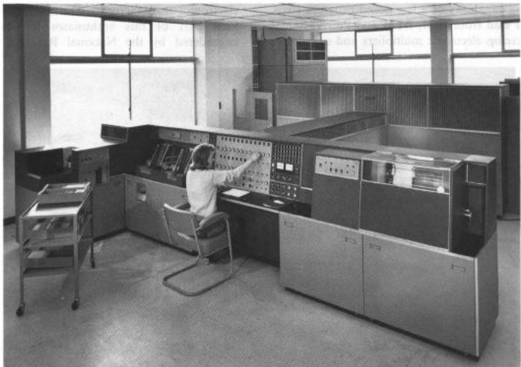
FIGURE 3. ICT 1301 (1962). The ICT 1301 was a medium-sized second-generation computer intended to compete with the IBM 1401. The price of typical installation was £100 000.
