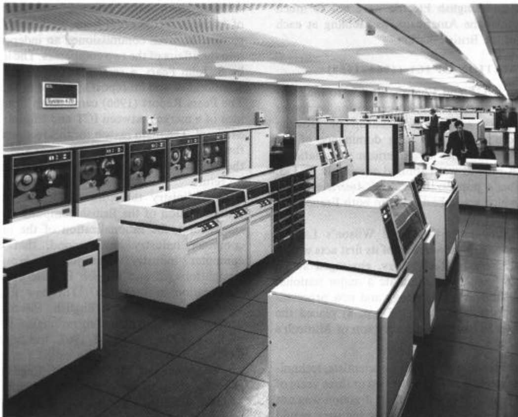
FIGURE 6. English Electric System 4-70. The English Electric System 4 was an IBM System/360 compatible range, based on the RCA Spectra 70 series. The large System 4 machines were particularly competitive in real-time applications.
