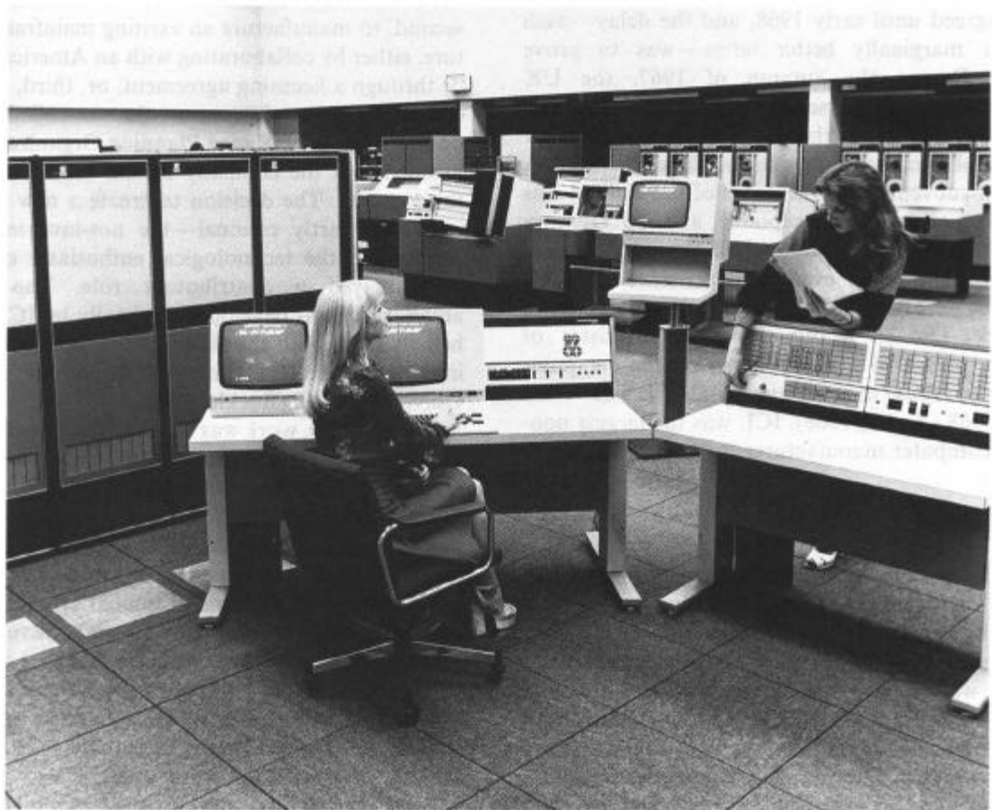
FIGURE 7. ICL 2900 series (1974). The ICL 2900 series was announced 1974. The new range was the most ambitious mainframe project ever undertaken in Britain and it remains the architectural base for ICL's current mainframes. The photograph—a publicity shot for the October 1974 launch—shows a mid-range model 2970.
