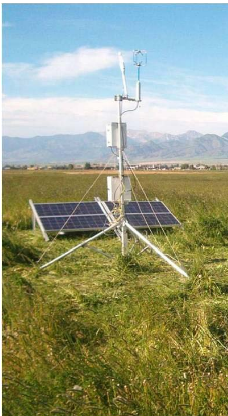
Figure 2.2.4. Example of a Eddy Covariance Tower System Source: (BSCSP, 2011d)
