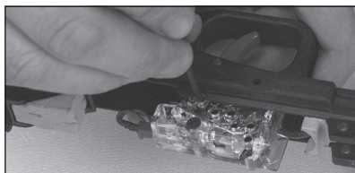
Figure 18: Adjust Trigger Over-Travel Cam
