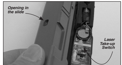
Figure 9: Take Up Laser Switch Must be Aligned with Hole in Slide When Reassembling Slide to Frame
