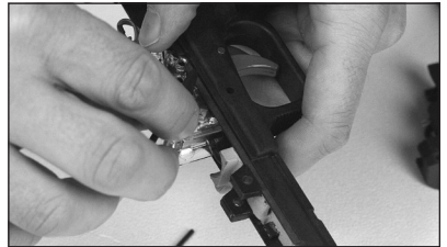
Figure 16: Adjust Initial Trigger Location Cam
