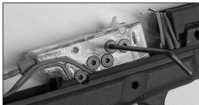
Figure 21: Loosen Sear Location Cap Screw
