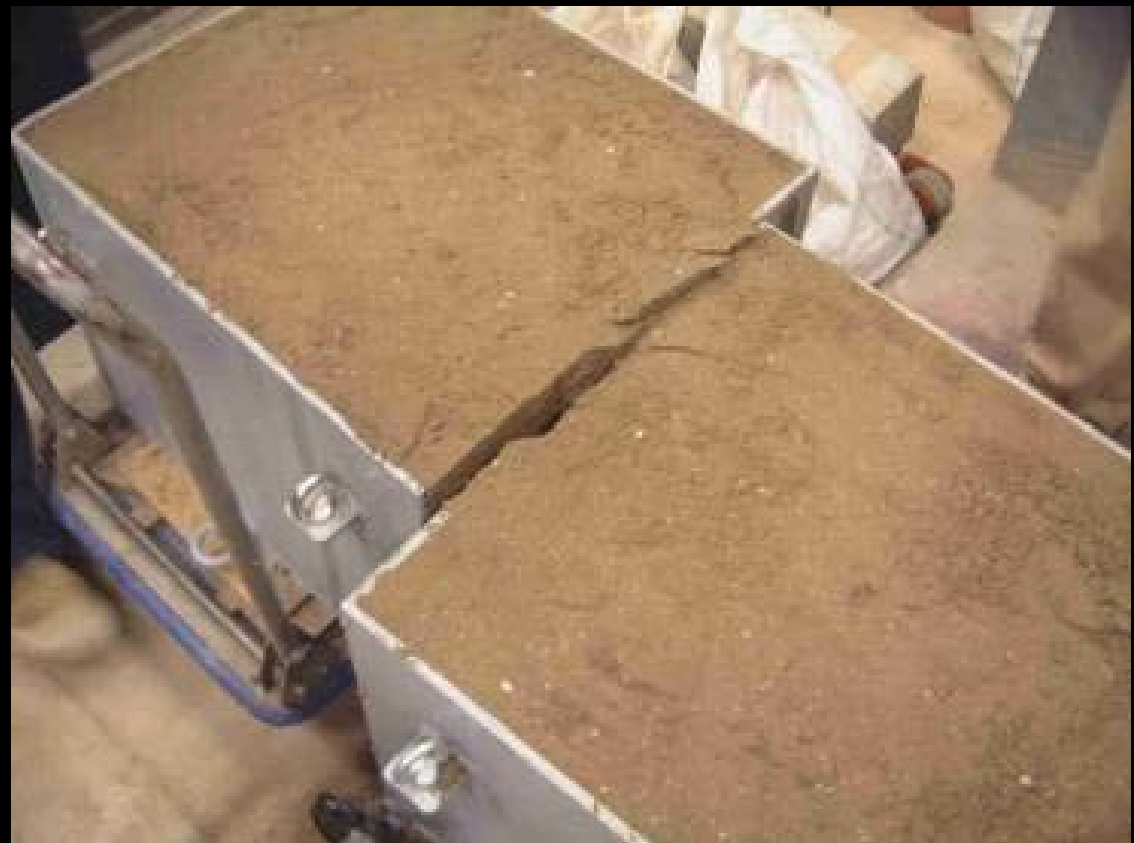
Laboratory scale modeling of strike slip faulting
