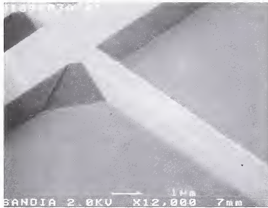
Lattice-plane selective etches provide reference features with atomically planar sidewalls
