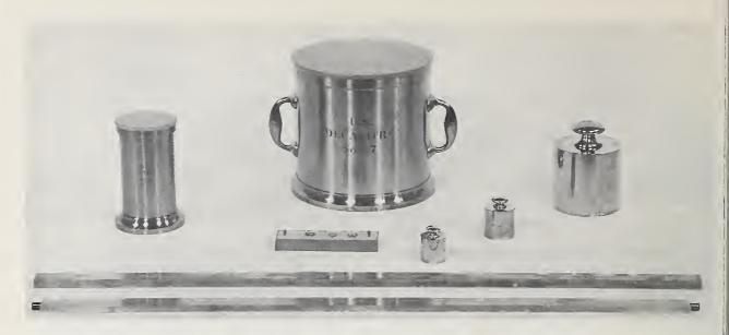
Metric standards of length, mass, and capacity, furnished to the States under the joint resolution of Congress of July 27, 1866.
