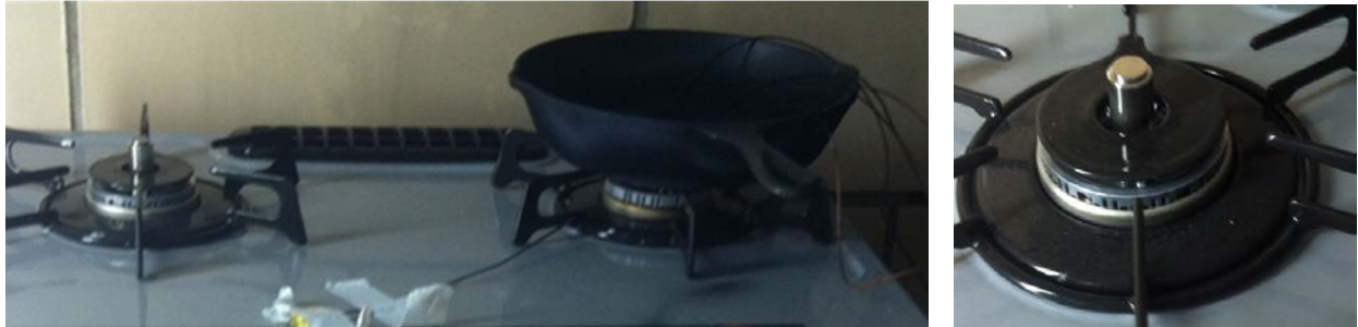
Figure 1 Gas cooktop with a spring-loaded bimetal switch protruding above the burner center (left). A close-up of the burner and sensor is also shown (right).
