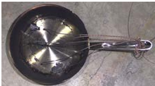
Figure 8. Black soot residue left inside Pan D (stainless steel) after Test 87 using Stove 6.
