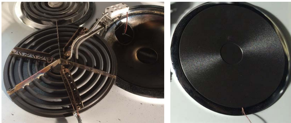
Figure 4 Bottom and top view of a retrofit technology composed of a thermocouple sensor to measure the temperature of the bottom of a metal plate that covers the coil heating element. Regulating electronics installed under the stovetop are not shown.
