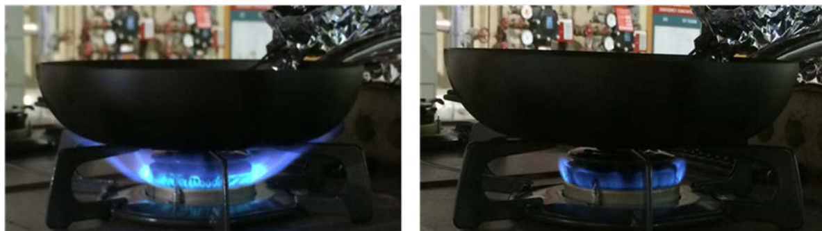
Figure 14 High (left) and low (right) fuel flow burner flame modes during experiment with dry Pan A on Stove 3.
