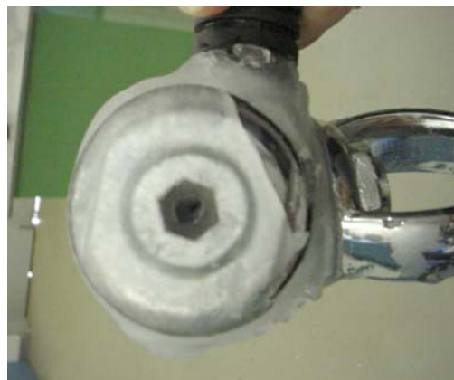
Figure 2. Close-up view of another first stage that functioned normally despite ice accumulation.
