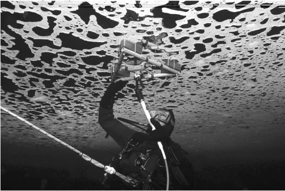
Figure 2. A DFO diver positions an ultra-sensitive light meter beneath 2-metres of sea ice in support of the Canadian Arctic Shelf Exchange Study (CASES).
