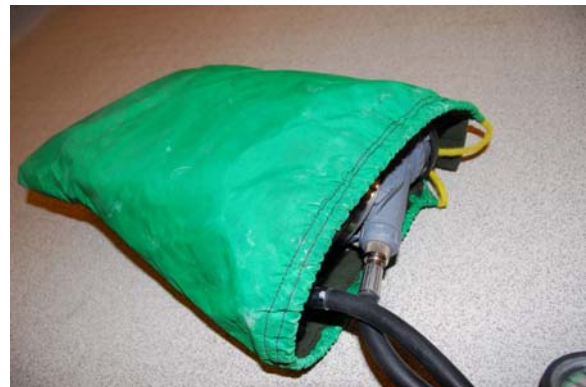
Figures 5a and 5b. The full-face mask is protected during transit out onto the ice with a lined wind- and water-proof bag (a). The mask is inserted into the bag (b) with the draw string tightened and kept in the bag right up to the final point of kitting up.
