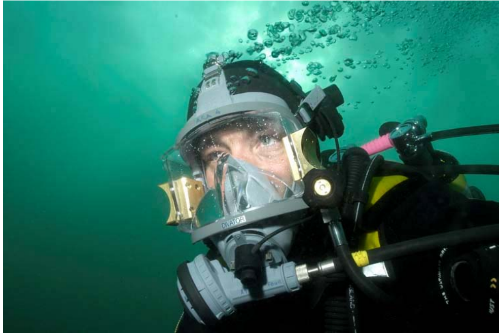
Figure 3. A close-up of the full-face mask configuration with manual bail-out side valve connected to a rear-mounted pony cylinder and push-to-talk voice communications with ear-mounted transmitter/receiver.
