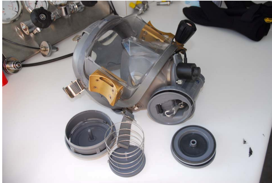
Figure 4. The between-dive routine maintenance for the AGA masks consists of opening up and drying the diaphragm cartridge which traps water easily.
