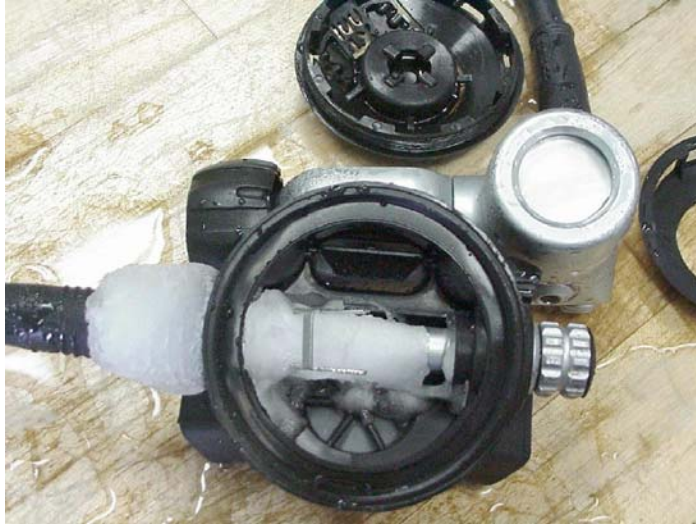
Figure 3. Second stage regulator that free-flowed because of ice accumulation around critical components.
