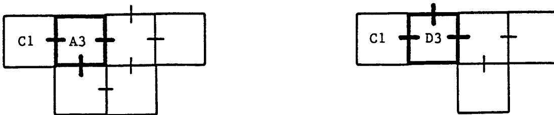
DIAGRAM 11.22. A3 (left): Space which provides direct access to a C1 space and has two or more additional accesses:
