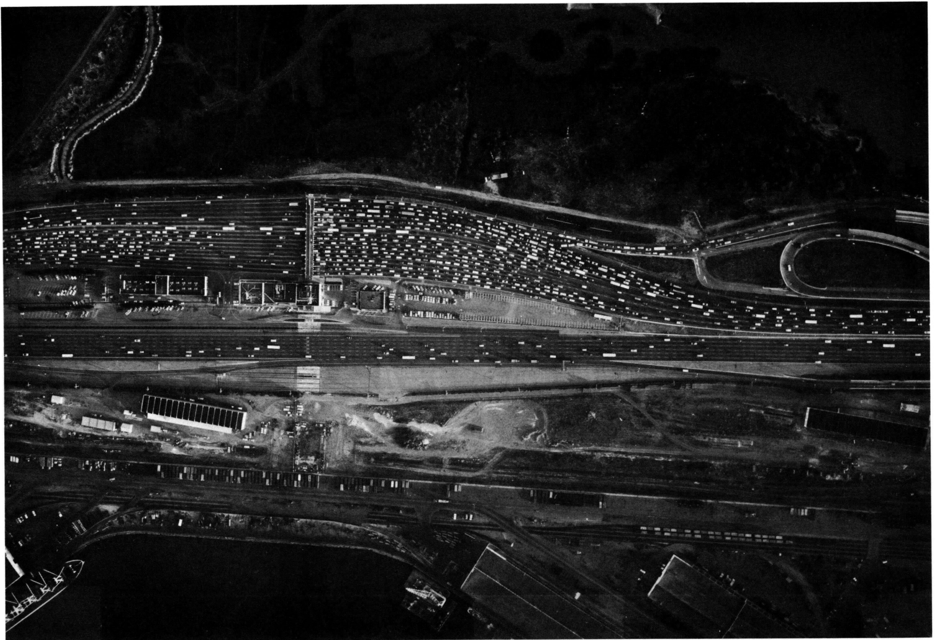
Figure B-47A. Bus bypass of car queues at toll plaza, San Francisco-Oakland Bay Bridge.
