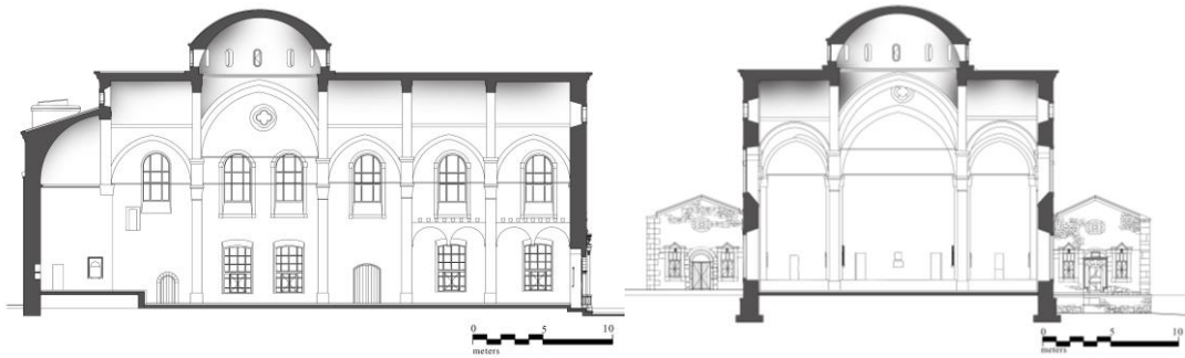
Figure 3.9 Section views of Surp Yerrortutyun Church from the central axis ( Source: reconfigured by the author )
