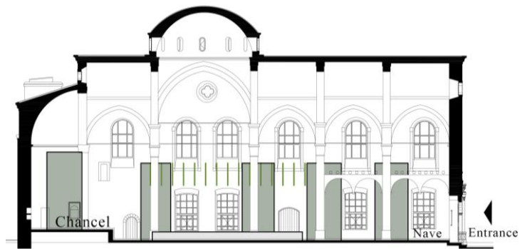
Figure 3.23 Proposal II in the Surp Yerrortutyun Church, plan and longitudinal section view
