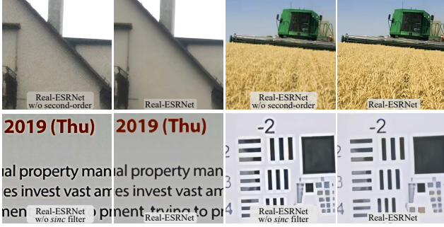
Figure 8: Top: Real-ESRNet results w/ and w/o second-order degradation process. Bottom: Real-ESRNet results w/ and w/o sinc filters. Zoom in for best view
