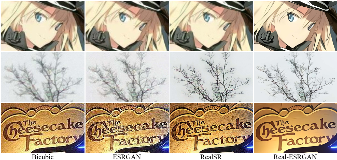
Figure 1: Comparisons of bicubic-upsampled, ESRGAN [48], RealSR [18], and our Real-ESRGAN results on real-life images. The Real-ESRGAN model trained with pure synthetic data is capable of enhancing details while removing annoying artifacts for common real-world images. ( Zoom in for best view )
