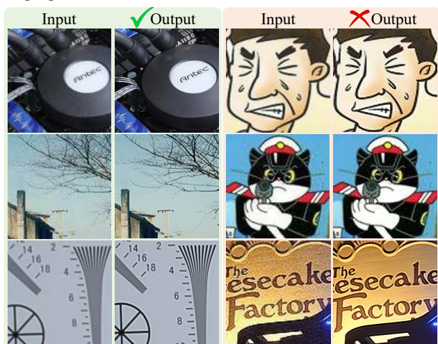
Figure 3: Models trained with synthetic data of classical degradation model could resolve some real samples (Left). Yet, they amplify noises or introduce ringing artifacts for complex real-world images (Right). Zoom in for best view
