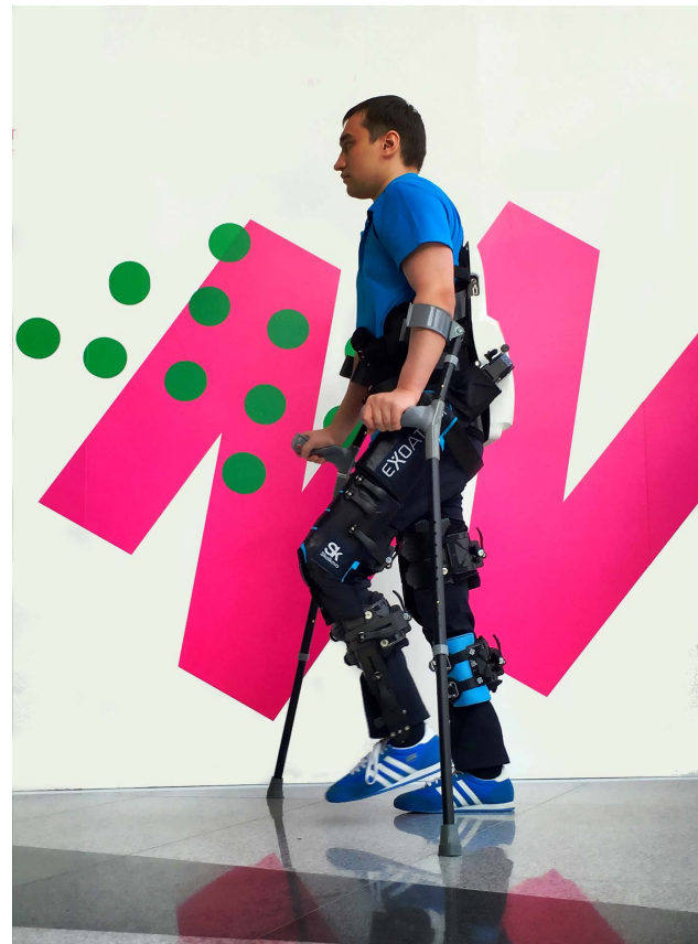
Figure 3. The ExoAtlet. This is an electrically actuated exoskeleton that assists patients suffering from leg paralysis. The ExoAtlet allows to set the stepping parameters and enacts several bipedal states, such as standing, walking on different surfaces and stepping over obstacles. Reproduced with permission from Ekaterina Bereziy, exoatlet.ru.
