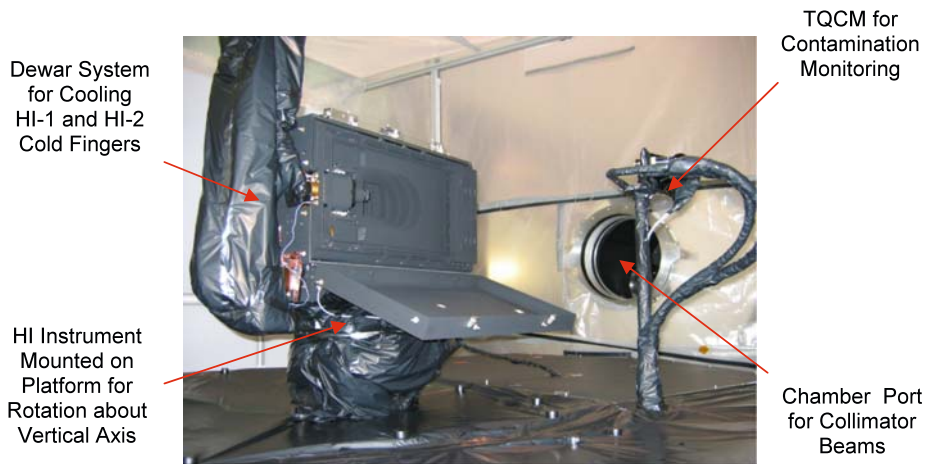
Figure 29 The HI-A instrument installed in a vacuum chamber at CSL for thermal vacuum qualification testing and optical calibration.
