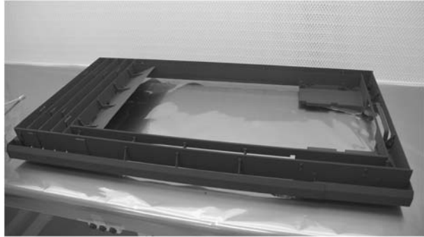
Figure 21 The forward and perimeter baffles support panel with the baffles installed.
