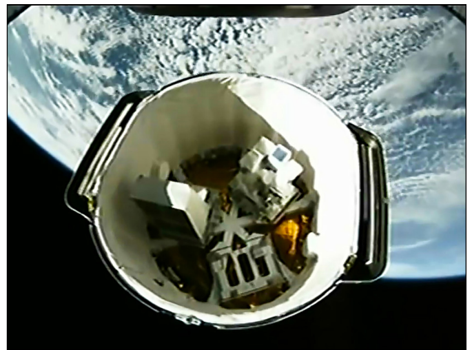
Figure 2. The Dragon trunk following separation from the SpaceX Falcon 9 second stage; clearly visible are the trunk payloads SDS at the 9 o'clock position and the Total & Spectral solar Irradiance Sensor experiment at the 1 o'clock position. The Flight Releasable Attachment Mechanism station at the 5 o'clock position was found empty for this flight. Credit: NASA
