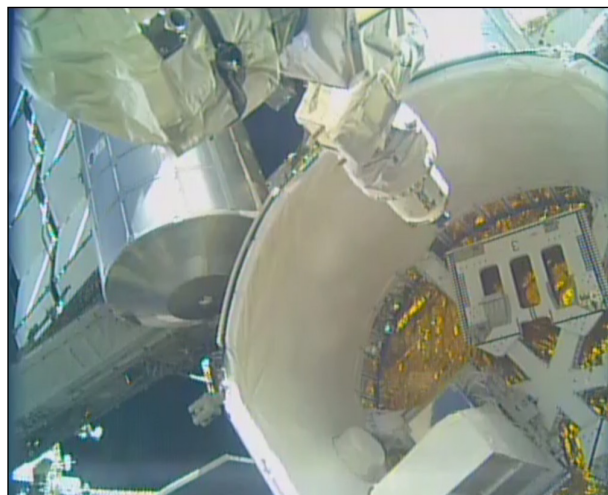
Figure 2. The SPDM OTCM enters the Dragon trunk.
