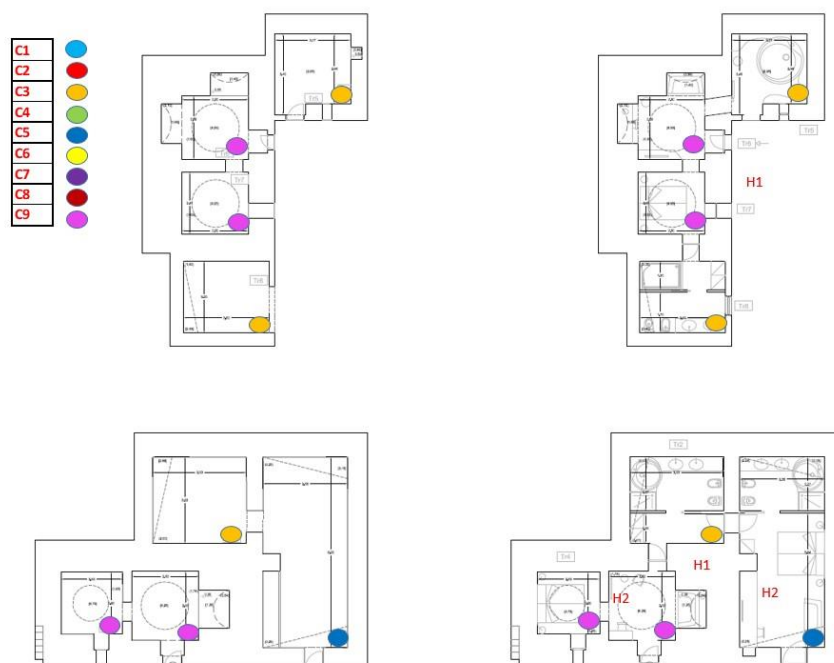
Figure 12. Trulli plan– Identification of basic and accessory cells (top) and reuse functions (bottom)
