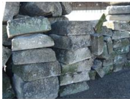
Figure 6. Stonework pieces from demolition.
