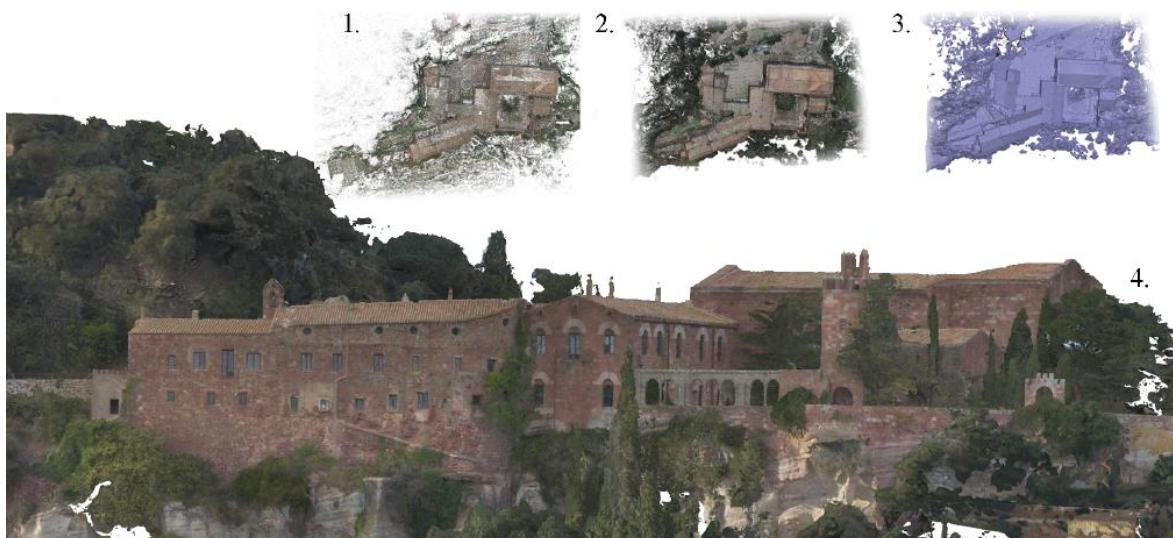
Figure 6. Photogrammetric model processing steps: 1. Sparse point cloud; 2. Dense point cloud, 3. Mesh, 4. Texture (acquisition and elaboration credits: Pietro Becherini).
