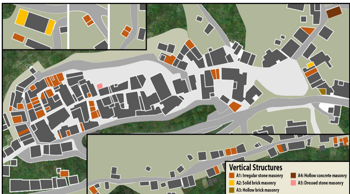
Figure 5. Mapping of vertical structures identified in the 51 building units. The colour represents the prevailing type found in the exterior walls, but more than one material is often present in the same unit – 2022 © Carlo Costantino
