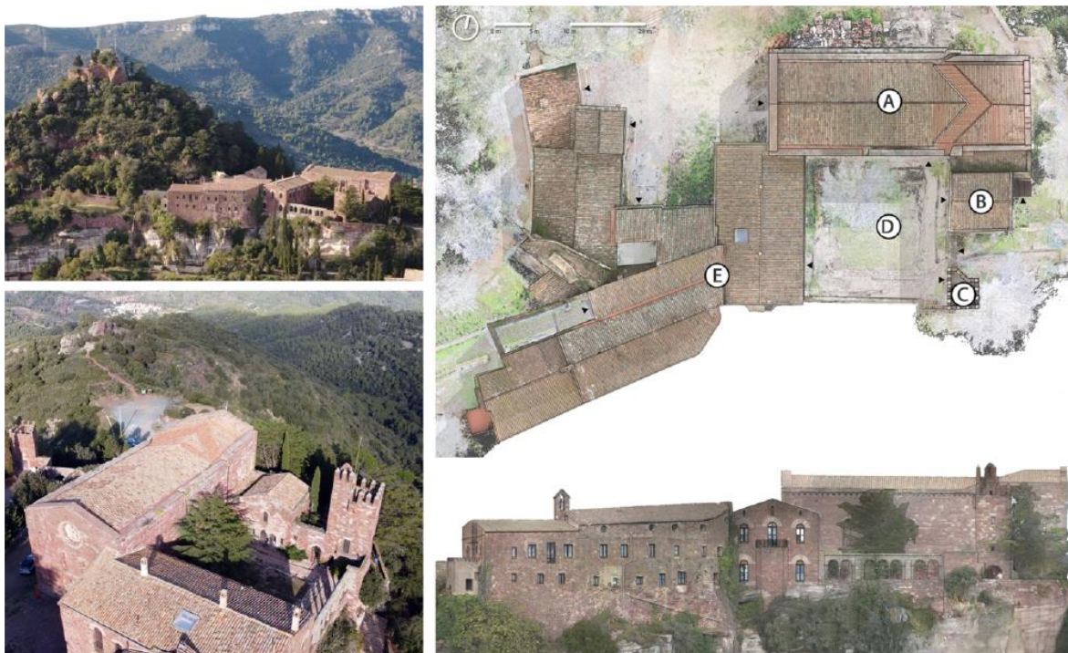
Figure 7. Aerial images of the complex acquired by Drone DJI Mini (credits: Pietro Becherini). On the right: a general plan of the complex with the indication of the main rooms: A - Church of San Miquel; B - Chapter room; C - South Tower; D - Cloister; E - Manor house. Below: south-east elevation with orthophoture.
