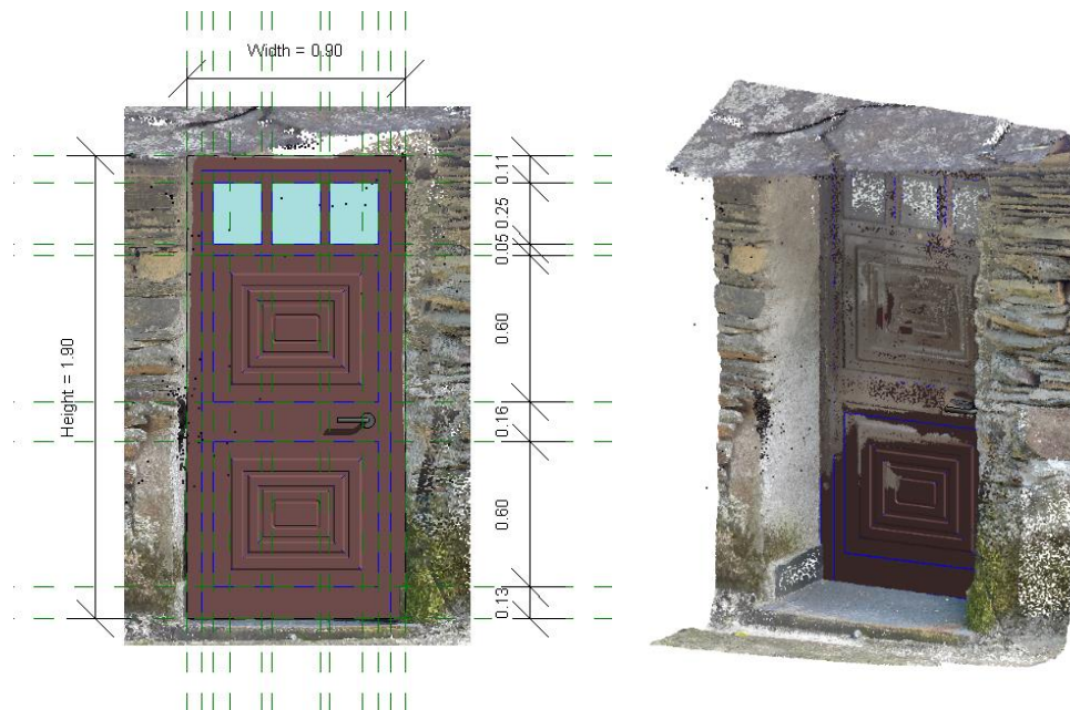
Figure 6. Modelling a door family on the point cloud (author's figure)
