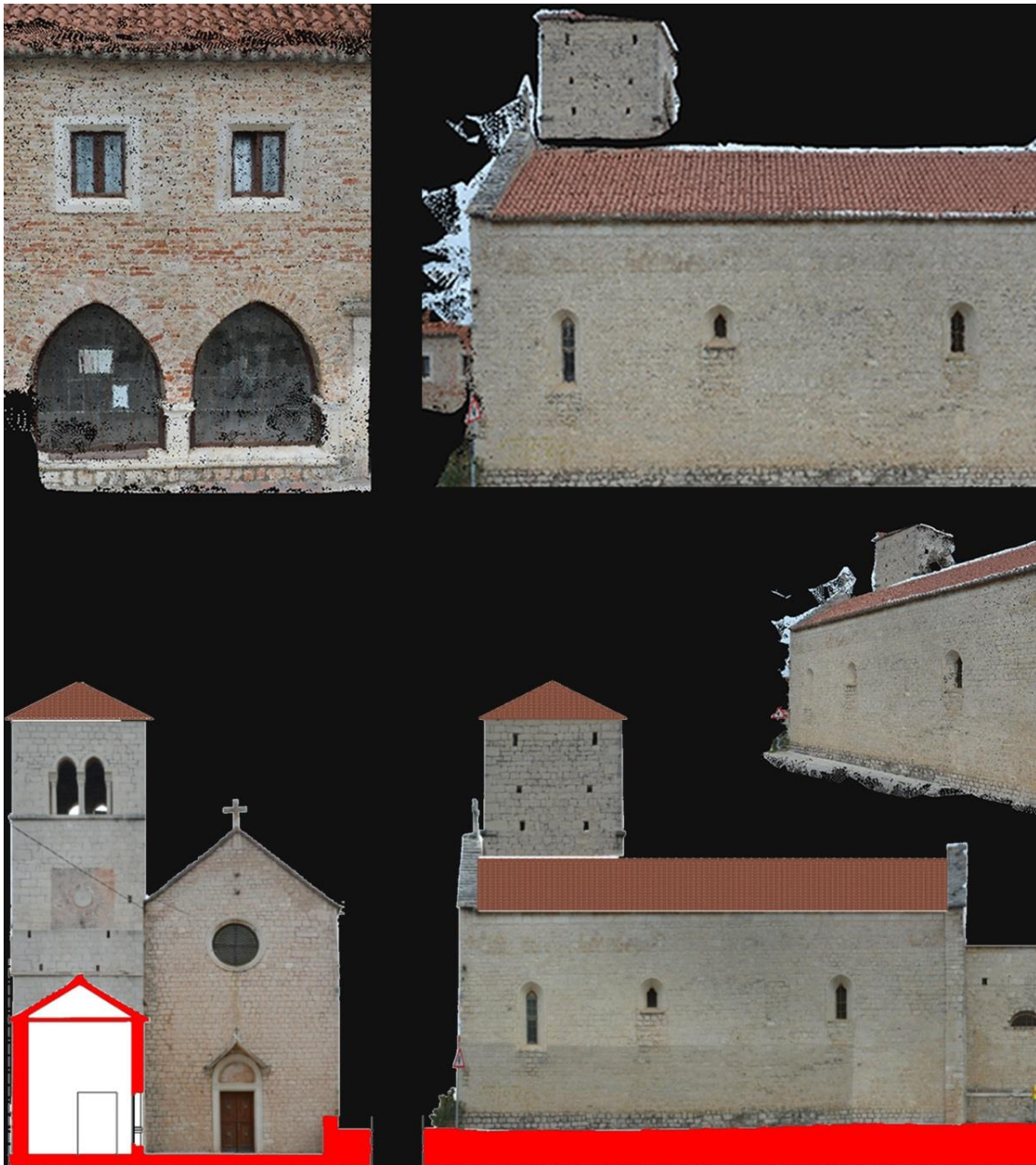
Figure 3. Processing of point clouds and orthomosaics from photogrammetric survey.
