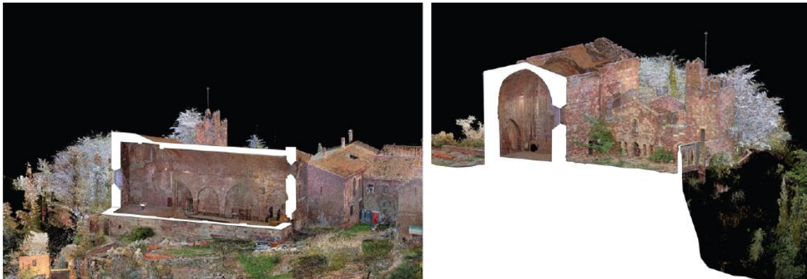
Figure 3. Perspective views of the complex obtained by setting section planes within the 3D point cloud.
