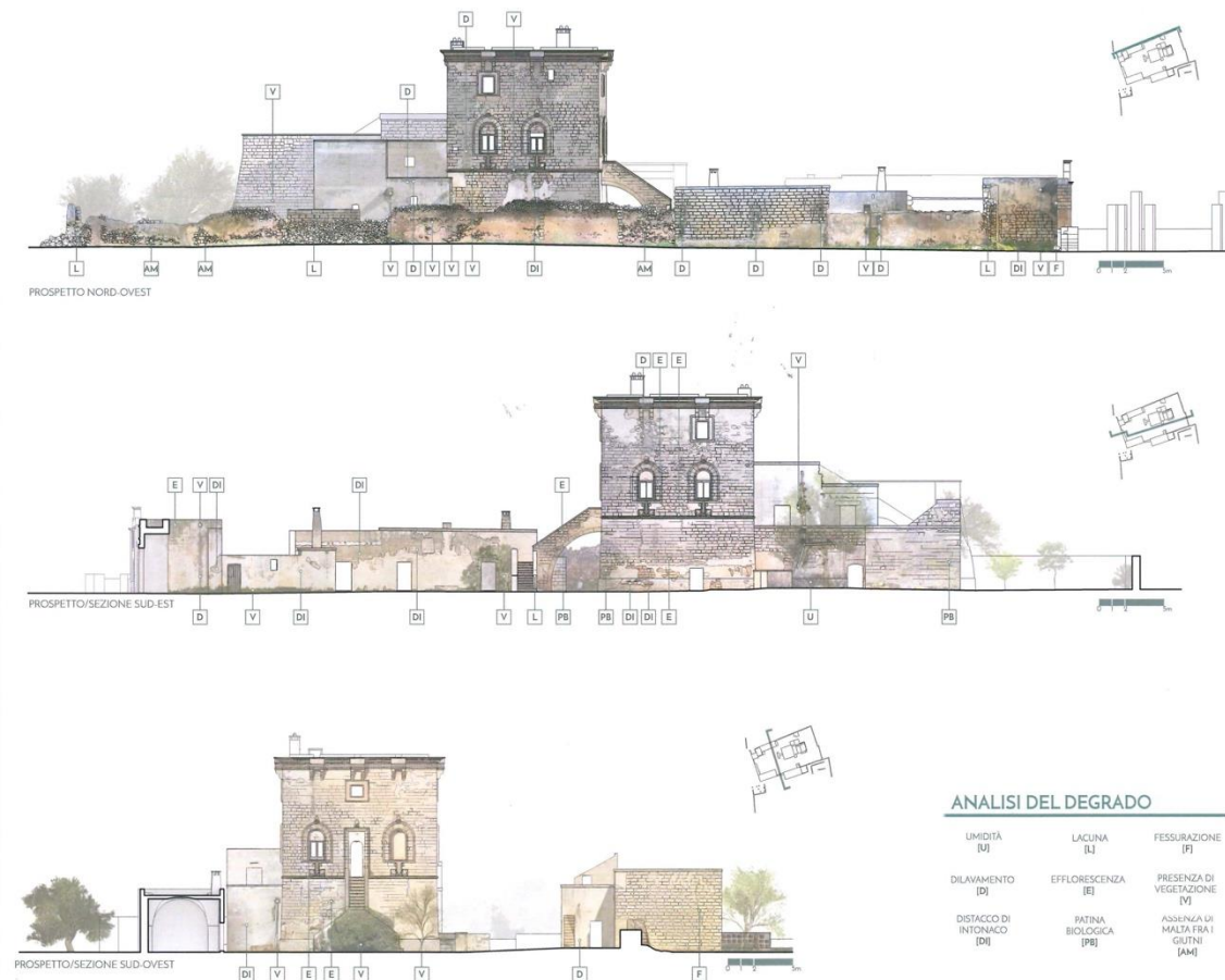
Figure 8. Trappeto farm, survey of the main forms of decay.
