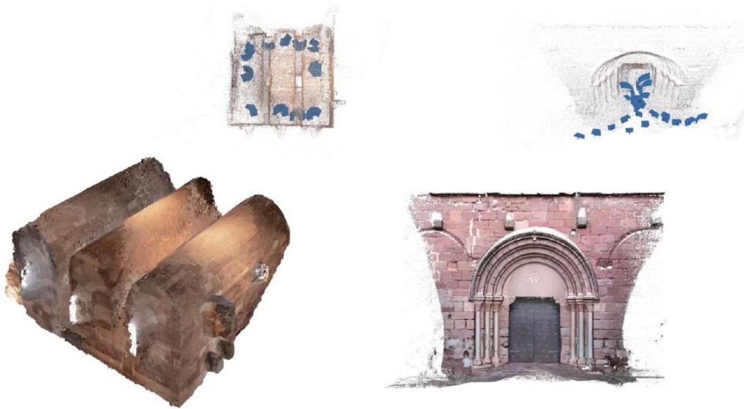
Figure 5. A photogrammetric model of the crypt (left), photogrammetric model of the church's portal (right). The acquisition schemes underline the different acquisition modes according to the object to be documented.
