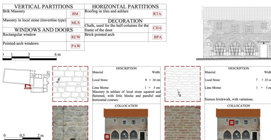
Figure 6. Geometrical-material survey of the hospice and cataloguing of masonry apparatuses.
