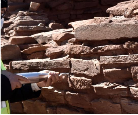
Figure 5. Schmidt hammer test.
