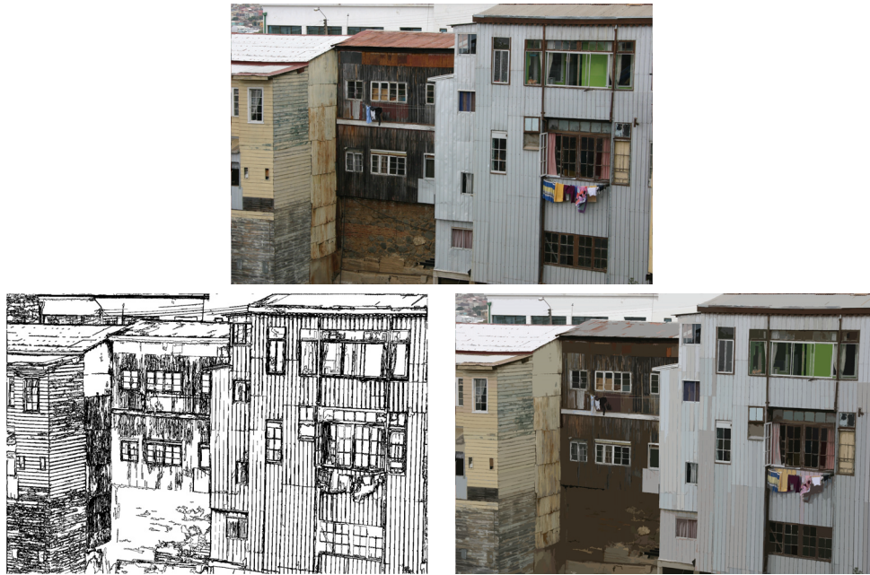
Figure 1. A digital image (top), its meaningful level lines (bottom left), and the sketch reconstructed only from these lines (bottom right). The texture has partly disappeared, but the geometric structures and the dynamics remain.
