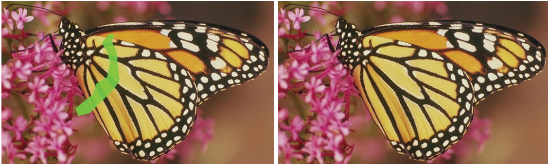
Figure 8. Top: original color image with an occluded zone. The transparency of the occlusion is for information only. Only the outer information is used for the reconstruction. Bottom: result after inpainting with straight lines [65] of each channel in a YUV representation.
