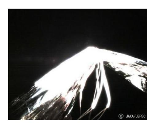
(PhysOrg.com) -- Japan's IKAROS has rolled out its solar sail, the first ever deployed in space. JAXA, the Japan Aerospace Exploration Agency, achieved the feat by rotating the craft rapidly and spinning the sail out by centrifugal force. IKAROS is the world's first solar-powered spacecraft.
