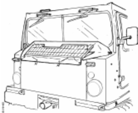
Fig 26. Plastic cover on air intake
