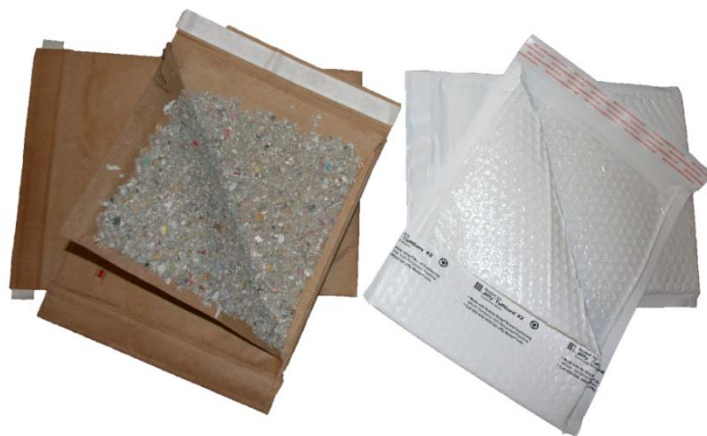
Figure 2: Kraft Paper and Newsprint Filled Padded Mailer and a LDPE Bubble Mailer
