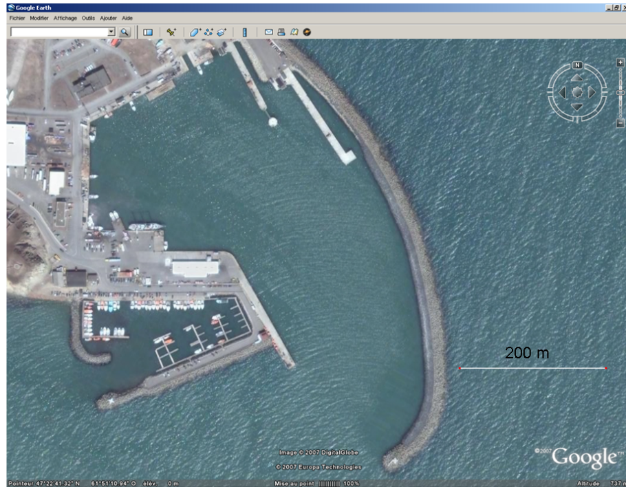
Appendix 9b. Made of concrete blocks and rockmound, the breakwater that protects the Cap-aux-Meules marina is used by gulls as a nesting site
