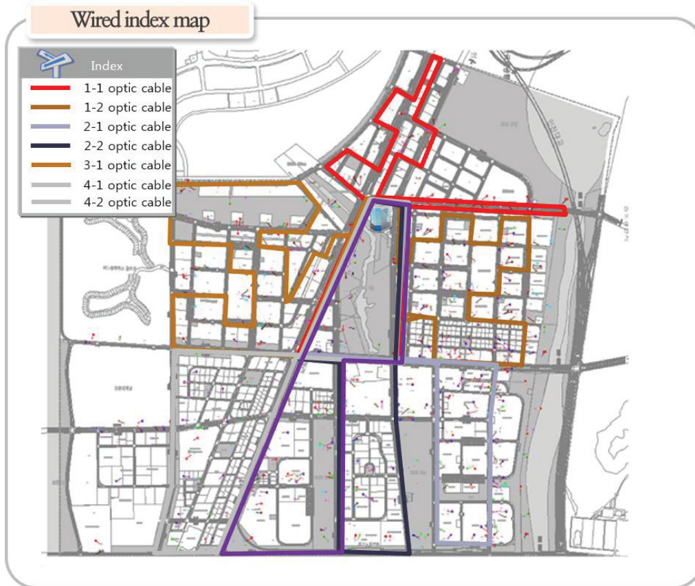
Figure 20 Fibre optic cable layout of Songdo U-city
