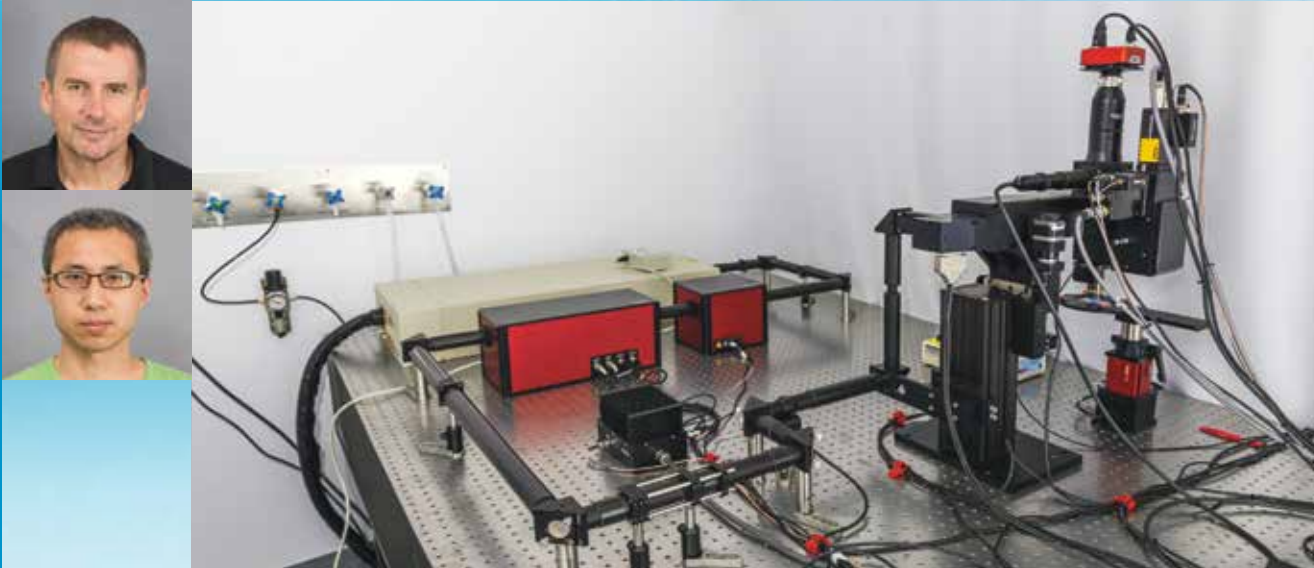
2015 laboratory members T-B: Barry Dickson, Kai Feng. Image: The Thorlabs microscope for fast volumetric activity imaging, modified for cell-type-specific activity perturbation experiments.
