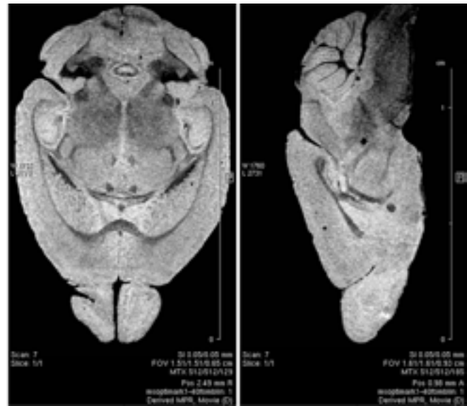
▲ 3D-spin echo of mouse brain. The acquisition parameters are TR/TE= 1500/13ms, 1 scan, acquisition time ~2.5h, at 117 \times 140 \times 280 \mu\text{m}^3 resolution using the 16.4T scanner.
