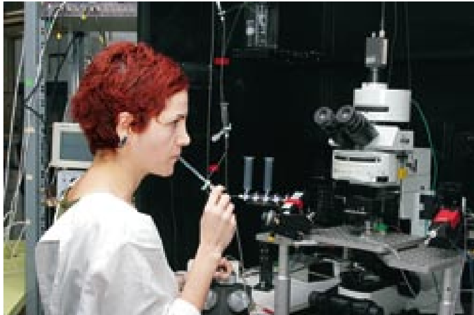
PhD student Sepideh Keshavarzi applies negative pressure to seal onto a neuron with a patch-clamp recording pipette
