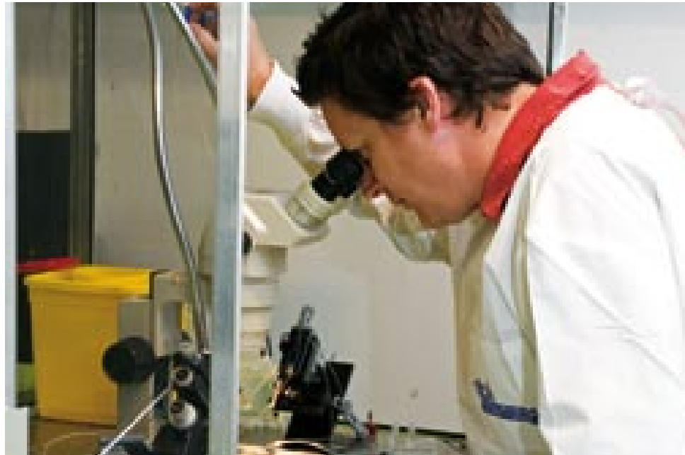
Postdoc Simon Nevin makes voltage-clamp recordings to test the effects of conotoxins on neurotransmitter receptors expressed in Xenopus oocytes
