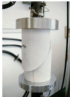
14 • Marble blocks of standard size and shape used for mechanical testing
