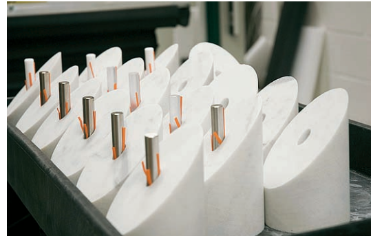
14 • Marble blocks of standard size and shape used for mechanical testing
