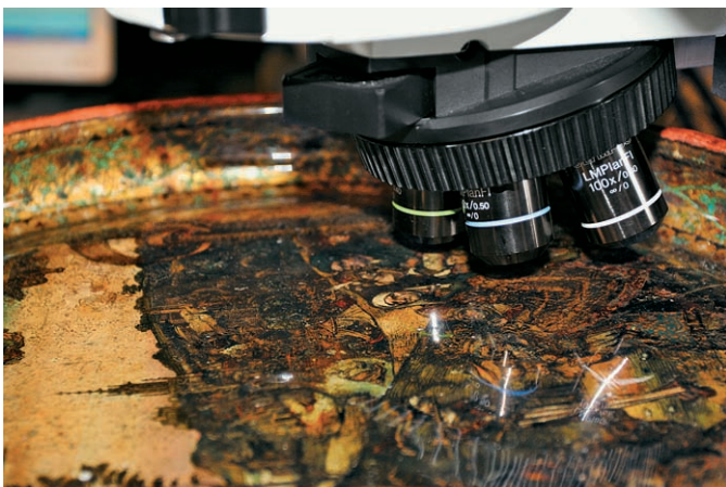
5 · Raman microspectroscopy being used to identify the pigments in a reverse-painted glass paten attributed to Hans Wertinger (German, d. 1533) and dated 1498 (free-blown glass with paint and metallic foils, diam. 14½ in. [36.9 cm]; The Metropolitan Museum of Art, The Cloisters Collection, 2008 [2008.278]). This technique can be used in a noninvasive way, without removing a sample from the object. A laser beam is focused on an area of the object (or a microscopic sample) through high magnification. The materials in the object interact with the laser beam, scattering it in all directions. Most of the light is scattered without changes, but a small number of photons undergo Raman scattering and can be detected at a longer wavelength than the original laser beam. The entity of the wavelength shift and the pattern of shifts (the spectrum) are characteristic of each molecule or crystal in the area of the object hit by the laser beam. In this case, the analysis was accomplished through a relatively thick layer of the glass, as the painted decoration was applied to the underside of the bowl.
