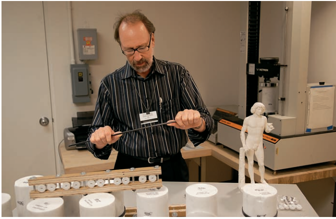
13 • To determine the best adhesive and pinning system to conserve a damaged marble sculpture, George Wheeler conducted exhaustive mechanical tests on sample blocks. In the foreground here is a scale model obtained by computer-aided machining following 3D laser scanning of the original sculpture: Tullio Lombardo (Italian, ca. 1455–1532), Adam , ca. 1490–95 (marble, h. 6 ft. 3½ in. [1.92 m]); The Metropolitan Museum of Art, Fletcher Fund, 1936 [36.163]). The virtual model was used for mechanical calculations and the scale model to test conservation approaches. In the background is the Instron tensile stress tester used to measure the strength of each adhesive and pinning combination.
