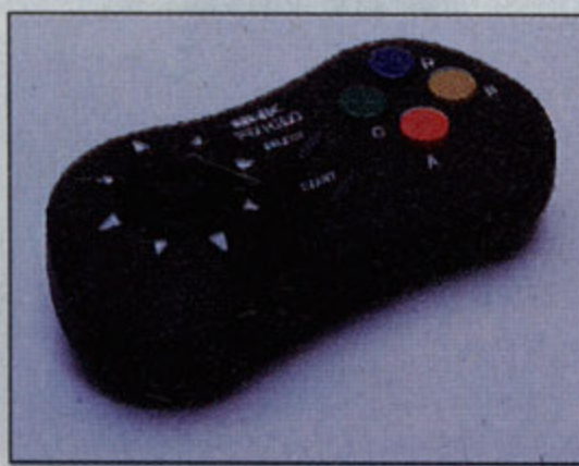
The control pad features the Neo•Geo's standard four buttons with a minijoystick thumb pad for directionals.
