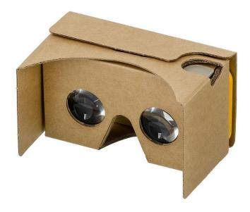
Figure 6. Google Cardboard can create the three-dimensional experience of virtual reality by using a very simple goggle setup with the use of a smart phone app.
