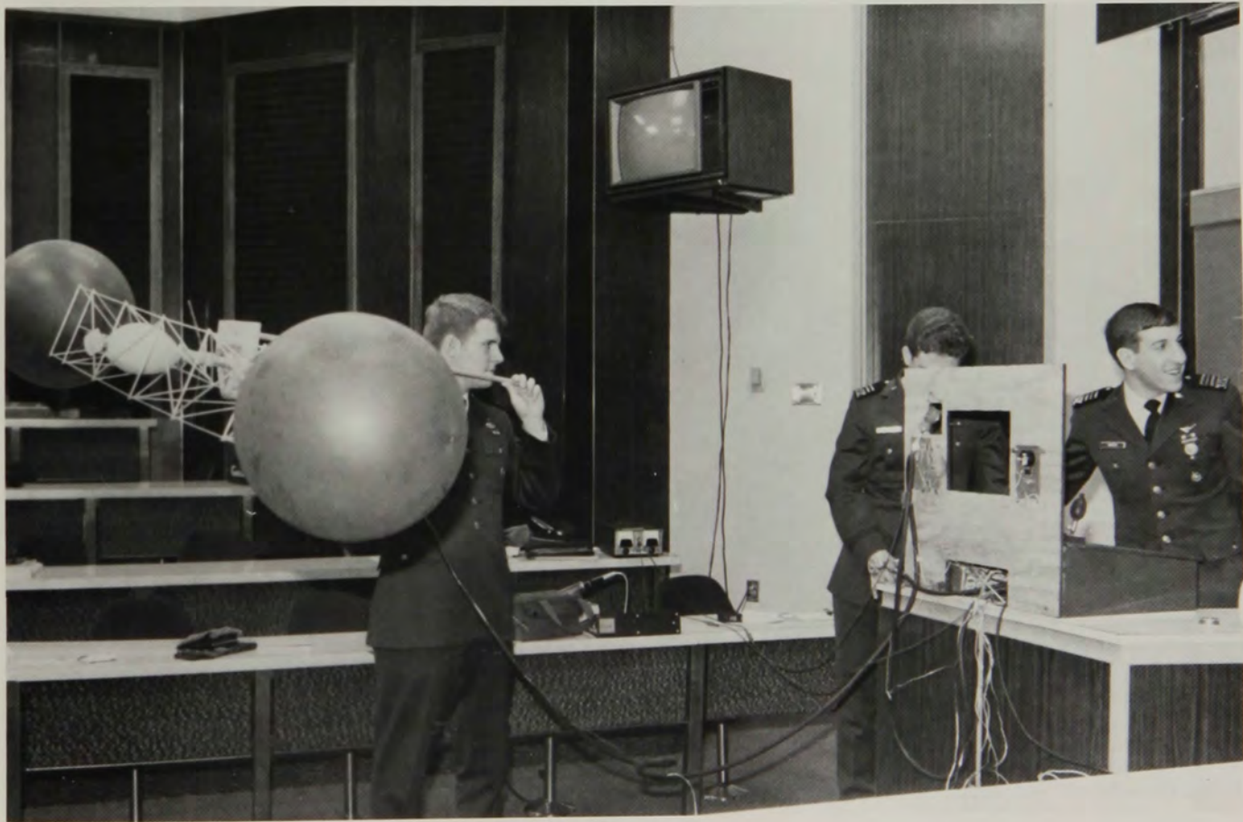
Caders Robert D. Beckel, Jr., Dirk M. Hutchison, and Michael J. Masucci work on the end effector model. Cader Beckel has inserted the end effector into the beam truss assembly. Cader Masucci has activated the controls which cause the end effector to inflate automatically to the proper size needed to grab the beam without structurally damaging the beam.
