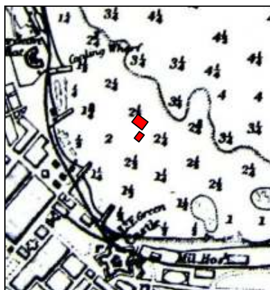
Figure 8: An extract from a plan showing the bathymetry of Table Bay in 1858, as surveyed by F. Skead R.N (see also Figure 2). Although the date on the chart suggests that it was prepared in 1858, some of the landmarks that have been included indicate that the map is probably from sometime after 1860. Depths in fathoms (1 fathom = 1.8288 meters). Sceptre Reef appears in front of the old Military Hospital at Woodstock.
