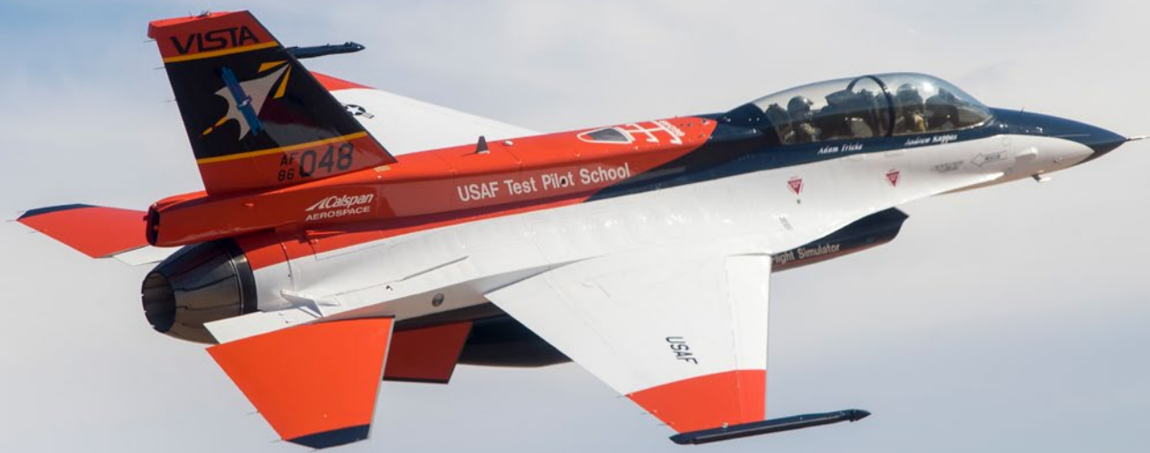
Loading their AI software into a specially modified F-16 test aircraft, like the one shown above, APL developers demonstrated that AI agents can control a full-scale fighter jet—and in the process gathered invaluable live flight data. (Credit: U.S. Air Force)
