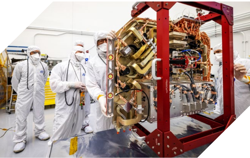
APL engineers work on Europa Clipper’s radio frequency (RF) panel, which is part of the larger RF module that houses the spacecraft’s telecommunications subsystem.
