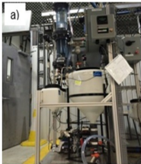
Figure 3-6: a) Ultrafiltration setup at Hydro-Québec and b) schematic of ultrafiltration bench system.
