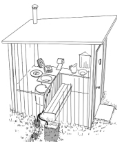
Urine-separating inset for dry closets.
