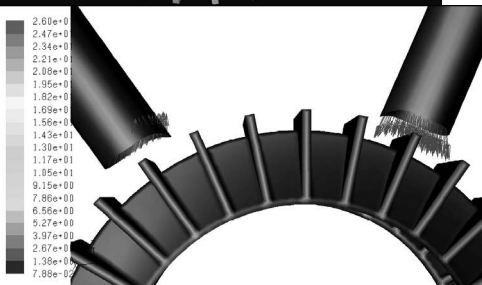
Velocity Vectors Colored By Velocity Magnitude (m/s) Jul 07, 2008 FLUENT 6.3 (3d, pbns, rke)
