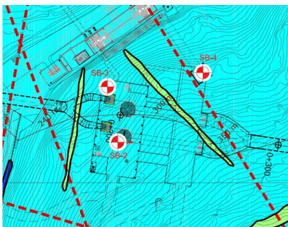
Figure 5. Geological plan at caverns level.
