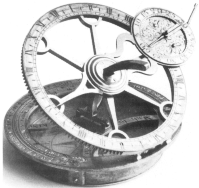
FIGURE 3: Universal Equinoctial Mechanical Dial by Thomas Wright.
