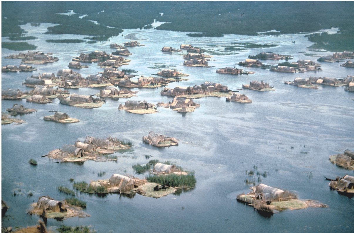
Fig. 5 - A typical marsh landscape. Villages are built on artificial floating islands by enclosing a piece of swamp, and filling it in with reeds and mud. For flood protection, more layers are added each year to strengthen the platform's foundation.
