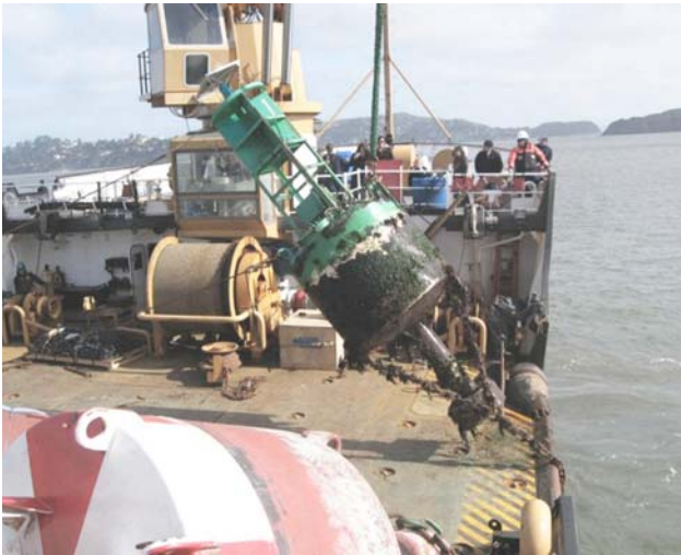
Figure 701a. Buoy with counterweight showing.
