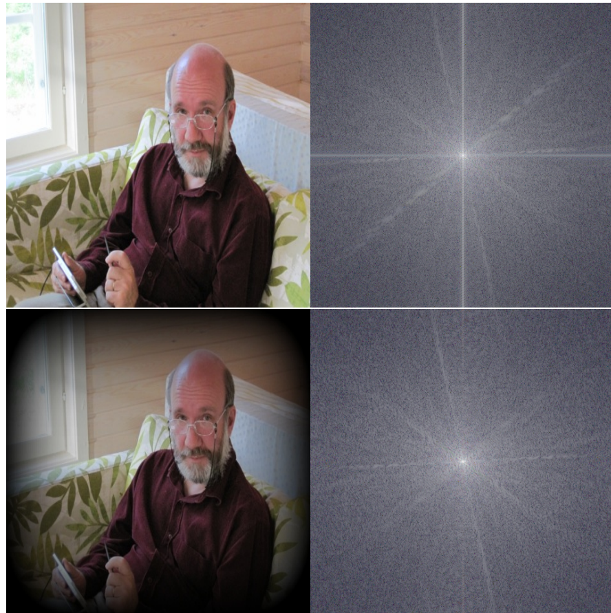
FIGURE 9.4. Example images for the FFT transform without (above) and with (below) tapering. The online FFT service from Watts (2004) was used. The images are greytone amplitude spectra |\mathcal{F}_{uv}| plotted with the origin u = v = 0 in the centre, see appendix C.
