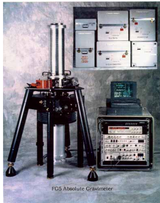
FIGURE 11.6. Absolute gravimeter of type FG5. Photograph United States National Oceanic and Atmospheric Administration (NOAA).
