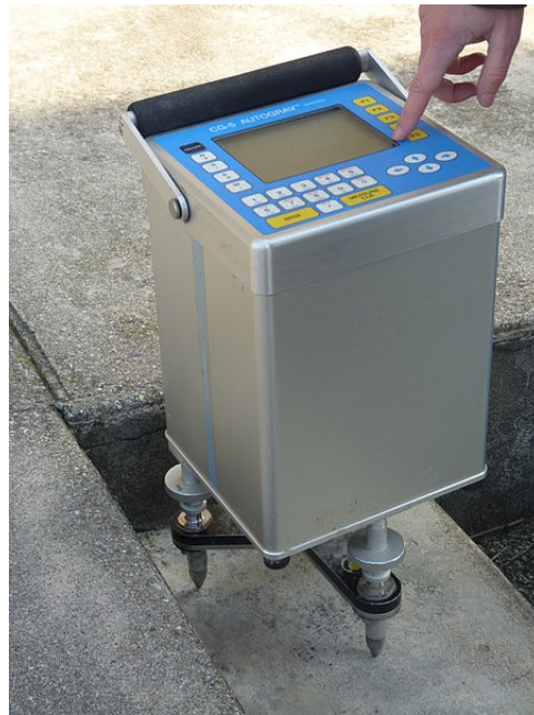
FIGURE 11.2. Autograv™ CG-5 spring gravimeter from Scintrex. Image Monniaux (2011) .
