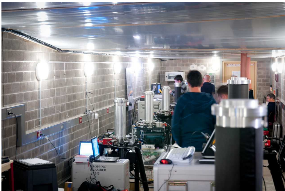
FIGURE 11.8. International intercomparison of absolute gravimeters in Walferdange, Luxembourg. Image courtesy © Olivier Francis.
