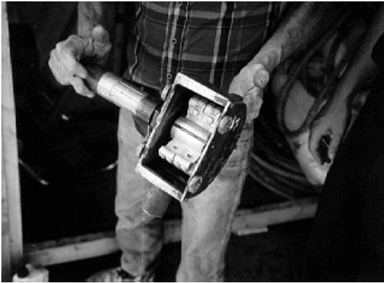
Figure 33. Close-up of the studded flaps mounted on the rotating head. To use the tool, it is held against the face of the iron member and as the studded flaps spin they “slap” the surface and “knock” the paint off the iron.
