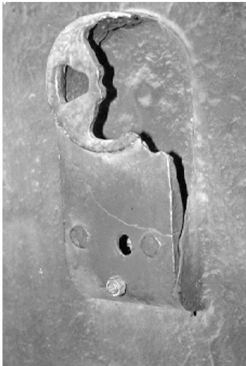
Figure 14. Nearly 30% of this ventilation shroud has been lost to two forms of abrasion: first, sand or grit blasting abraded away a majority of the material; second, human touch has smoothed the once rough surface.
