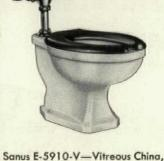
Sanus E-5910-V—Vitreous China, Syphon-Jet Closet, with elongated rim.  $1\frac{1}{2}$  " top inlet for flush valve, as specified. Projection from wall,  $28\frac{1}{2}$  ". (With round front, projection from wall,  $26\frac{1}{4}$ ".)
