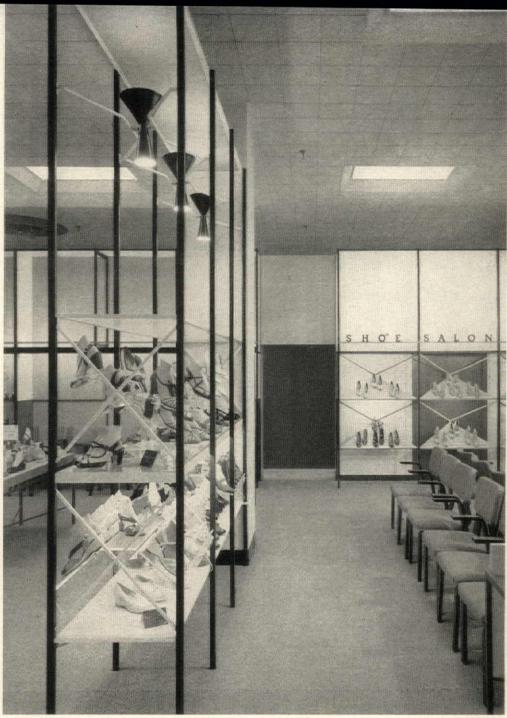
TWO-WAY FIXTURES of various sizes and shapes incorporate shelving, panels of wire mesh, cross-bracing and built-in lighting. Both wire mesh and cross-bracing are used decoratively as well as structurally. Frame is usually sprayed a dark color; other elements
