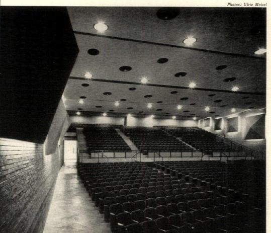
"stadium" balcony that does not separate the audience sharply in half. Acoustical "pyramids" of varying sizes and depths were introduced to break up reverberations between parallel walls, conceal indirect background lighting. Roof and hung acoustical ceiling is carried on 84' steel trusses.
