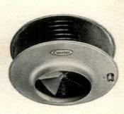
CARRIER VERTICAL UNIT HEATER. For highly efficient down-blow heat distribution from high ceilings. Avail-able for steam or hot water. Choice of heating patterns in twenty sizes from 30,000 to 576,000 Btu/hr.
