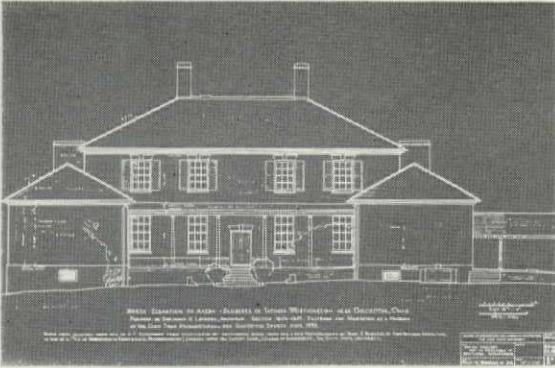
PHOTOGRAMMETRY enables Ohio State Architect Perry Borchers (standing, left) to produce orthographic drawings of historic buildings, such as Benjamin Latrobe's Adena, built in 1807, near Chillicothe, Ohio. Borchers is applying photogrammetry in a basic research project as well, attempting to measure subtle movements of structures under varying thermal conditions.
