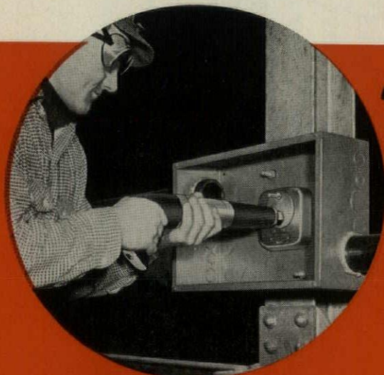
Split-Second "Nailing" To Concrete or Steel with OMARK DRIVE-IT Tools.
