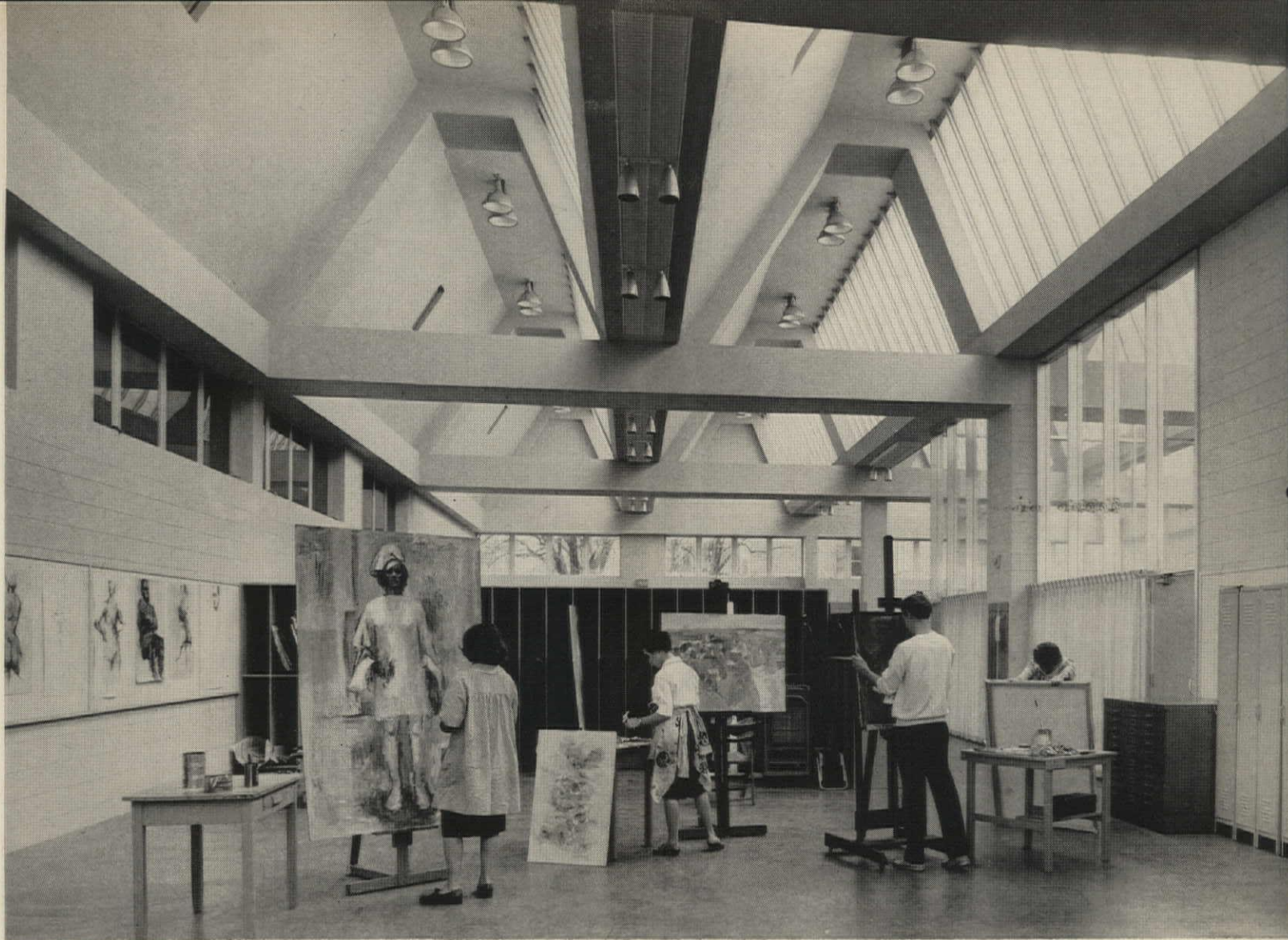
Studio space indoors (above), exterior (below). Beam 10 feet above floor level is hung from frame of building by panels over doors.
